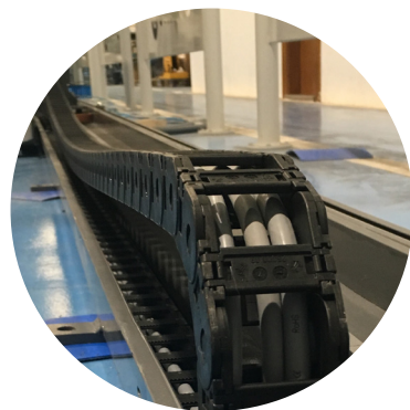
Detail of carriage guide for full pallets
